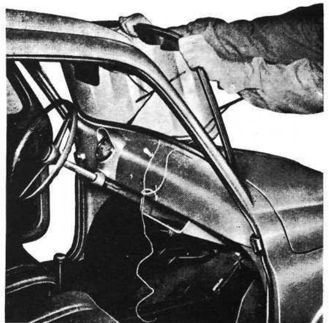
FIG 12:7 Positioning the windshield after tilting wiper blades
