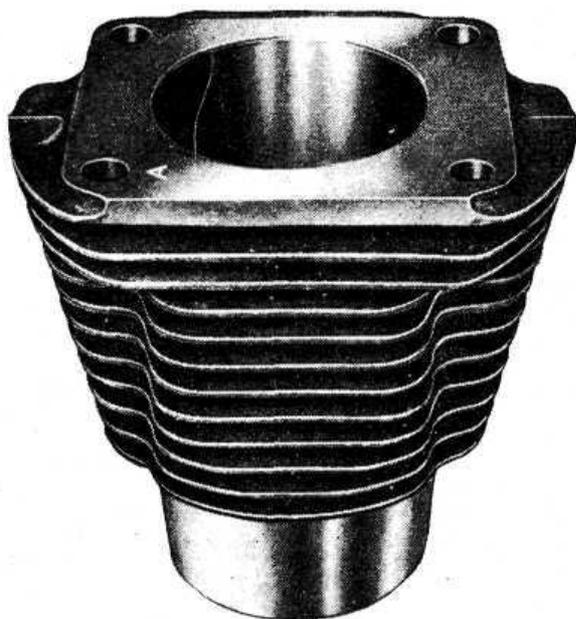
**FIG 1:21** Finned cylinder. Letter A stamped on cylinder indicates the class to which cylinder belongs, as referred to its inside diameter
