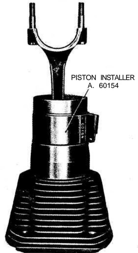
FIG 1 :28 Piston installer A.60154
