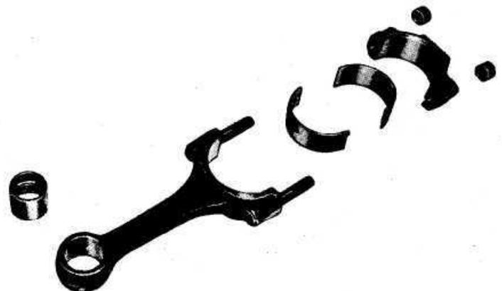
FIG 1 :29 Connecting rod components
